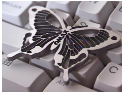
Typical results when machined with the OMAX MAXJET 5 MiniJet Nozzle
